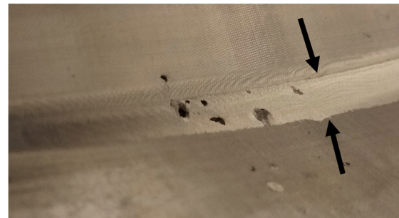
Figure 17. Closeup of surface deviation in a fillet on the mold face. The arrows point to the change in surface finish that occurred when the ball endmill entered the fillet and deflected.
