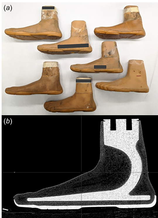
Fig. 7 The recovered feet appear to be undamaged after months of use. (a) Photo of the seven feet recovered from participants personal identifying participant information has been covered by spoilers. (b) CT scan of a randomly selected recovered foot showing no damage to the inner keel.
