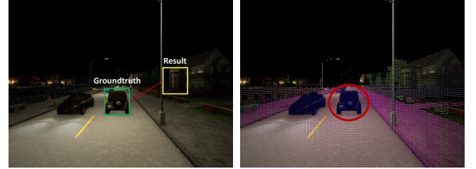
Figure 12: Effects of sensor fusion on attack results. Although the object tracker is hijacked (left), the original object still registers on the LiDAR (right, circled).
