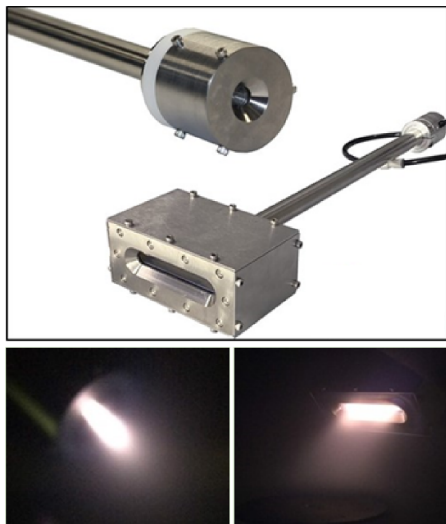
Figure 9. Round and linear (78 mm effective length) single beam plasma sources and discharges.
