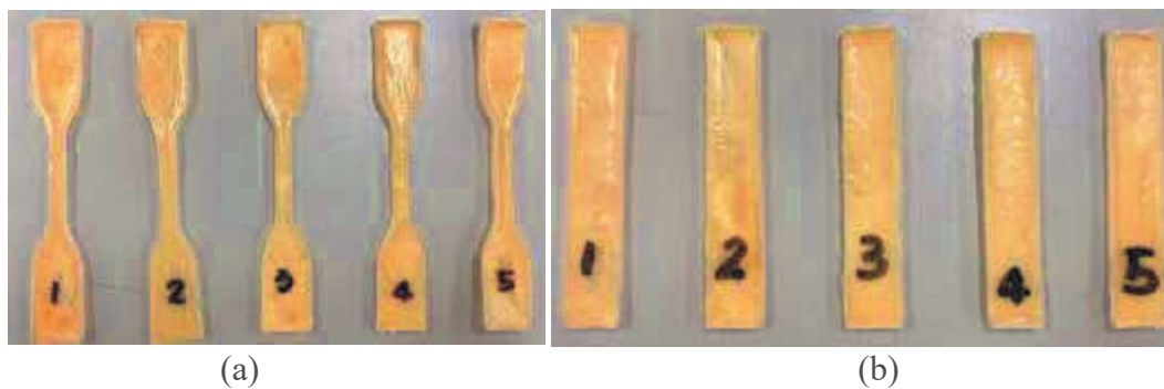
Figure 2. Pure Elium samples made for (a) Tensile, (b) Flexural tests.
