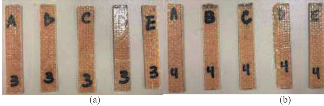
Figure 7. (a) 3-ply, and (b) 4-ply Elium resin infused and thermo pressed woven jute specimens.
