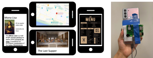
Figure 3: (a) Example templates used by the mobile application. Allows the broadcast system to specify how content will be rendered on the users’ devices. (b) Mobile phone equipped with UWB.
