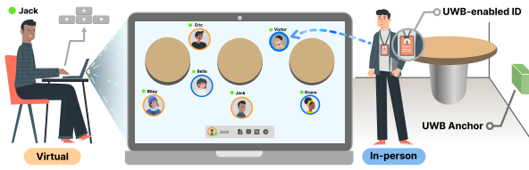
Figure 1: Real world participants appear in the virtual space. Their location is tracked using UWB localization as they move around in at the conference venue. Virtual participants use arrow keys to navigate the virtual space.
