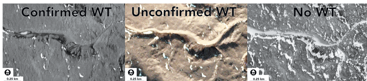
Figure 3. Example of classification of water track or wetland activity. At left, in the terrain-corrected image, dark linear features are interpreted as water tracks. In the center panel, darkened pixels may be water tracks and/or ponded soil moisture wetlands; however, because the image could not be terrain corrected, it is considered “unconfirmed.” At right, no water tracks are present in the terrain-corrected image.
