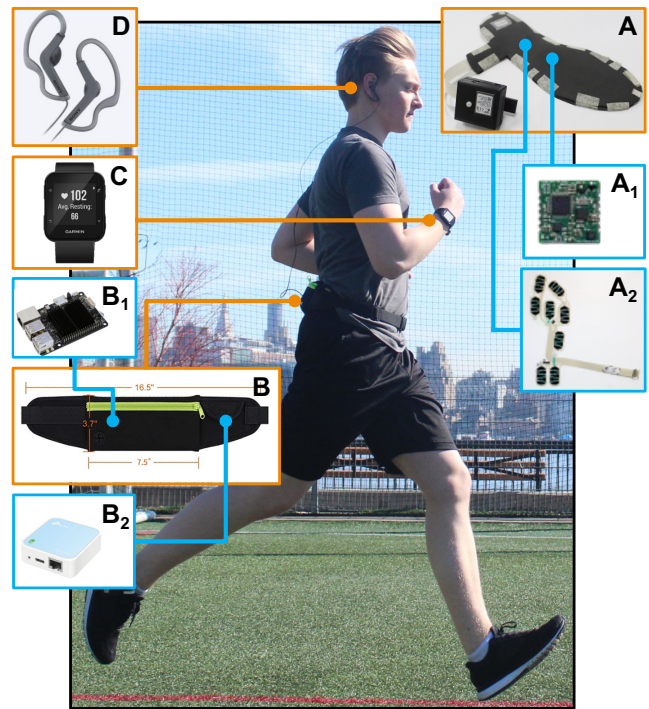
Fig. 1. The CyberCoach consists of (A) Custom-engineered instrumented insoles ( SportSole ) featuring embedded IMU ( A_1 ), FSR array ( A_2 ), and logic units; (B) a running belt with embedded single-board computer ( B_1 ), Li-Po battery, and miniature Wi-Fi router ( B_2 ); (D) sport earbuds to deliver the auditory feedback. An off-the-shelf running watch (C) was used for comparison, but it is not part of the proposed system.
