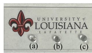
Figure 9. Image of a coated glass slide after annealing with droplets of (a) 20 wt % caustic, (b) water, and (c) 37 wt % HCl.
