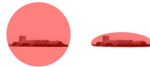
Figure 3. Ray Bounds. NeRF++ (left) samples within a unit sphere centered within and enclosing all camera poses to render its foreground component and uses a different methodology for the outer volume complement to efficiently render the background. Mega-NeRF (right) uses a similar background parameterization but models the foreground as an ellipsoid to achieve tighter bounds on the region of interest. It also uses camera altitude measurements to constrain ray sampling and not query underground regions.
