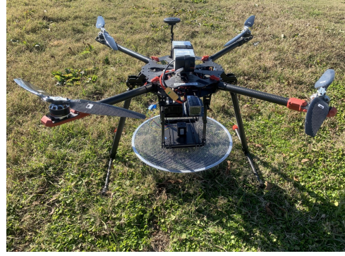
Fig. 3. Experiment with rotating phones, placed on the ground and under a quad copter. Both phones with ground plate spin at the same speed. A picture of the drone step up is shown.
