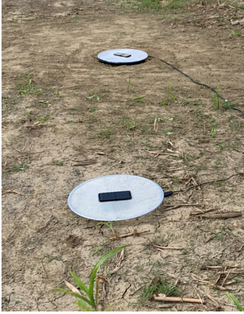
Fig. 2. Experiment with rotating and stationary phones, placed on the ground. The phone in the back rotates with a constant speed while the one in the front stays stationary towards a certain direction
