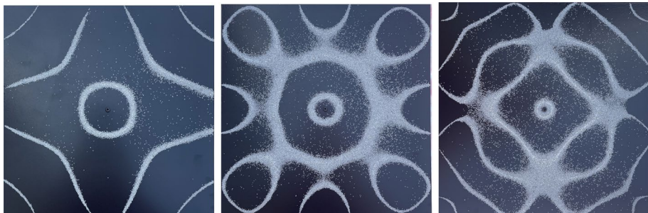
Fig. 1 The sand patterns of a plate which vibrates at three different frequencies (photos taken by authors)
