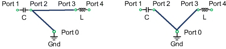
Fig. 7. The same (partial) circuit with two different topology representations with different edges.
