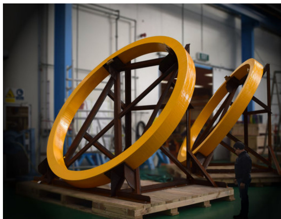
Figure 27. Photo of cyclotron coils built by Buckley Systems, Auckland NZ. These coils are 3.3 m diameter, ours are 4.95. The proportions are about the same as ours. Notice the person in lower right.
