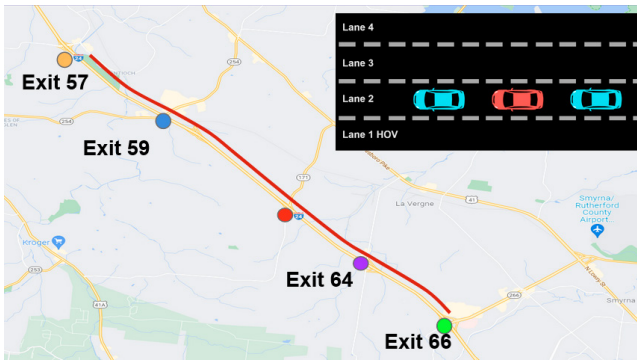
Fig. 1. The driving route for the 2021 experiment (medium-scale) on I-24 Southeast of Nashville. All 11 cars drove in lane 2 during the Westbound direction. AVs (red) were between manually driven cars (cyan) that were instrumented to measure the AV's effect on traffic.
