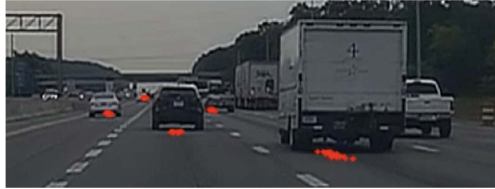
Figure 1. Five vehicles being tracked simultaneously with use of multi-object tracking algorithm associating CAN data.
