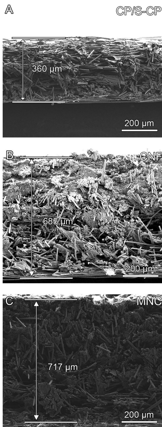
Figure 5. Thickness of different carbon electrodes measured by the cross-section SEM images: (A) CP and S-CP, (B) CNF, and (C) MNC.
