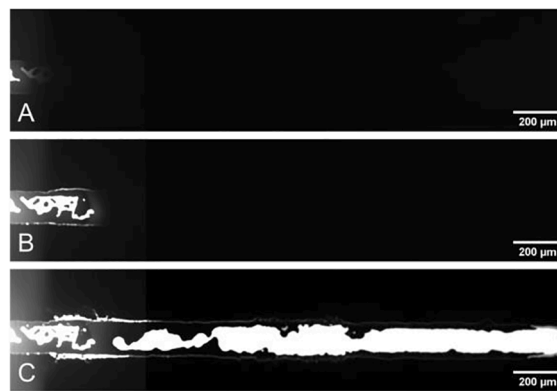
Fig. 10. Time series of discontinuous displacement in a nanoscale channel. (A) 30 min, (B) 150 min, (C) 12 h.
