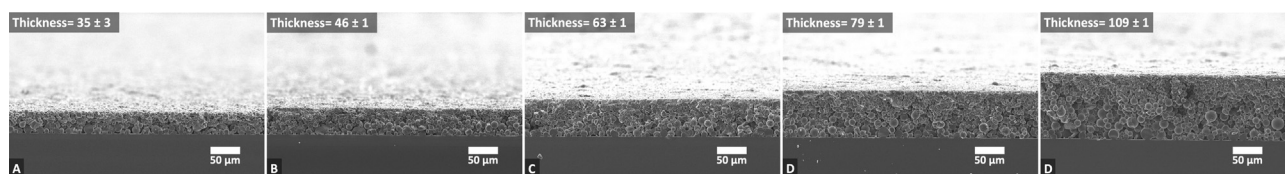
Fig. 2. SEM images of porous coatings with thickness labelled. Images show uniform thickness of coatings.
