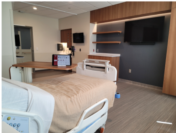
Figure 1: A smart patient room in the NRH with a hospital-furnished iPad running the smart room app. Each patient room has lights, blinds, thermostat, television, and soundbar that can be controlled with the smart room app installed on a hospital-furnished iPad or on a personal device. In several rooms, the door can also be controlled.
