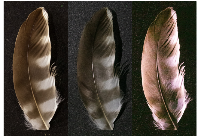
Fig. 5. Sample of photographs captured with the dome under varying illumination. Note the changes in specular highlights on the microstructures.
