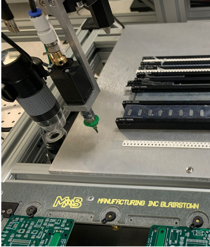
FIGURE 2: VACUUM NOZZLE PLACING COMPONENTS ON PCB IN THE NEXUS SYSTEM
