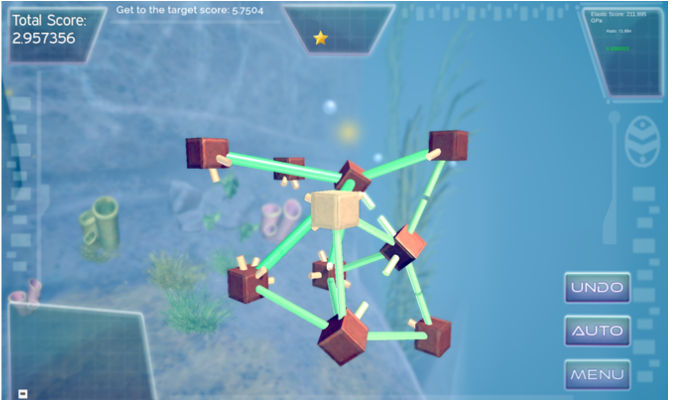
Figure 3: Full game view of a 3D grain boundary network in-game. Players are able to maneuver through the 3D space to manipulate the orientations of grains, and receive visual feedback on how their changes affect both the local properties of the incident GBs and the effective macroscopic material property. The view shown here represents current version of the HCG. Players participating in the study were given a visually simplified yet functionally identical version.
