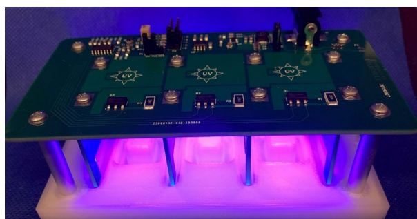
FIGURE 2 LED source over 3D printed (PLA) test fixture with three isolated sample wells
