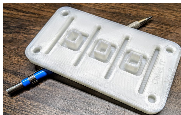
FIGURE 1 3D printed polylactic acid test fixture with three light-isolated wells for performing triplicate experiments
