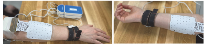
Fig. 1: Two wireless OT Bioelettronica high-density sEMG 8 \times 8 grids attached to the extensors (top) and flexors (bottom) of the forearm for gesture prediction.
