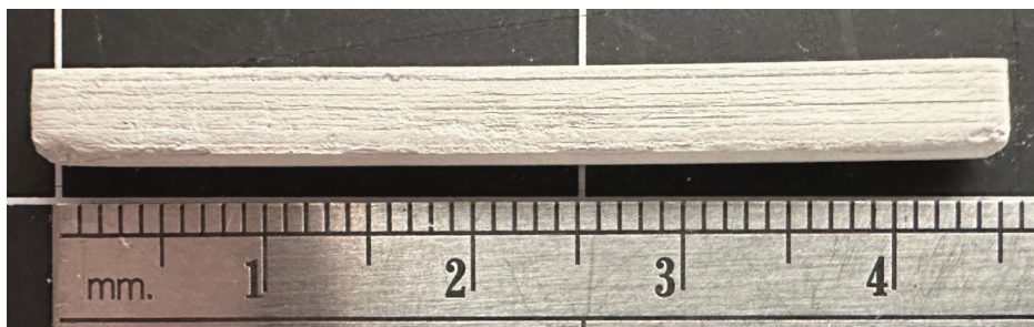
Fig. 5 Green \text{Si}_3\text{N}_4 beam after water debinding and drying.
