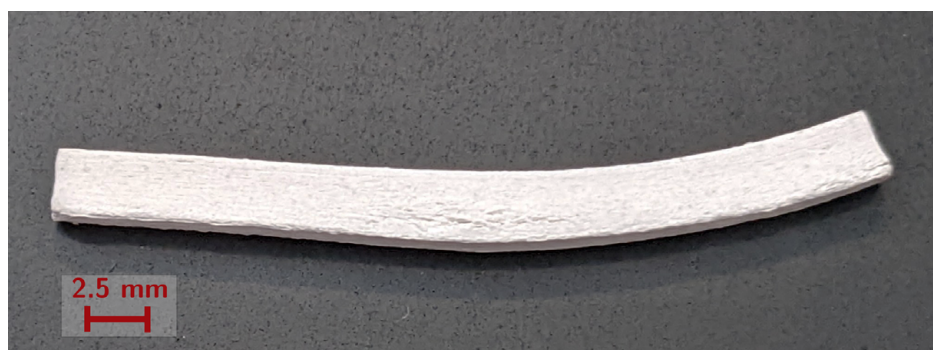
Fig. 7 Sintered beam with visible layer lines and warping due to poor interlayer adhesion
