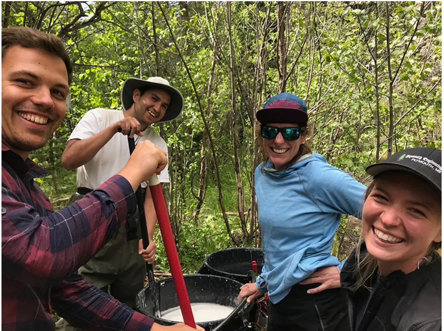
Students (left to right) Stefan Klingler, Ian Gambill, Jackie Randell, and Anna Marshall mix salt into water for an in-stream tracer test at Little Beaver Creek, a tributary of the Cache la Poudre River in northern Colorado. The tracer allows scientists to study the role of logjams in controlling surface water movement. Credit: Kamini Singha
