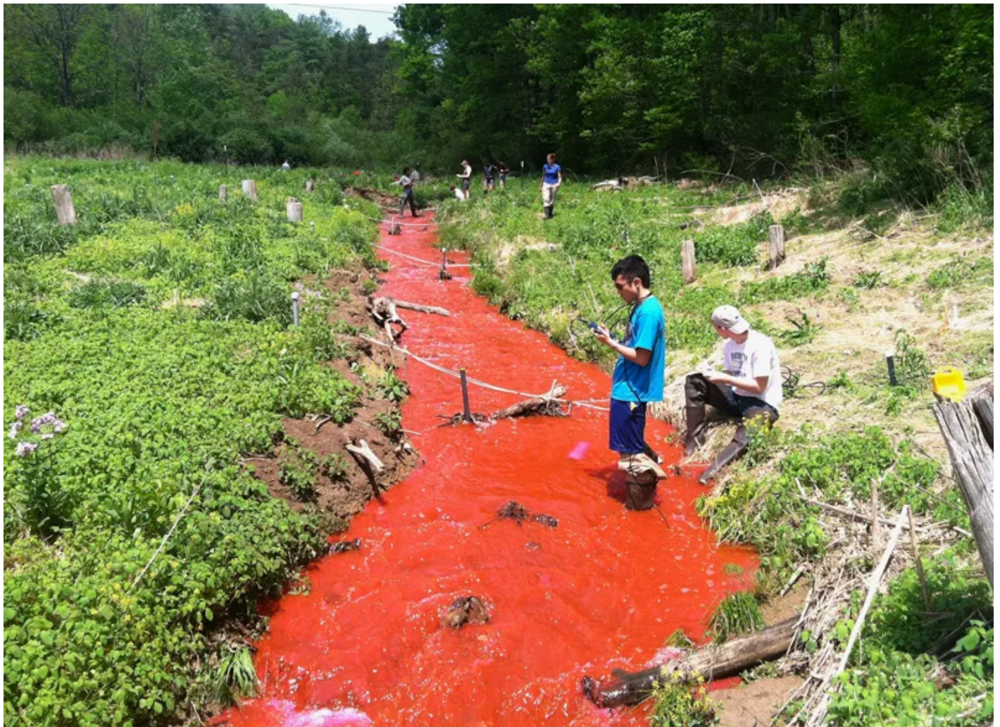
Students perform a dye test, which helps them to estimate groundwater–surface water exchange near the Susquehanna Shale Hills Critical Zone Observatory in Pennsylvania. Credit: Kamini Singha
