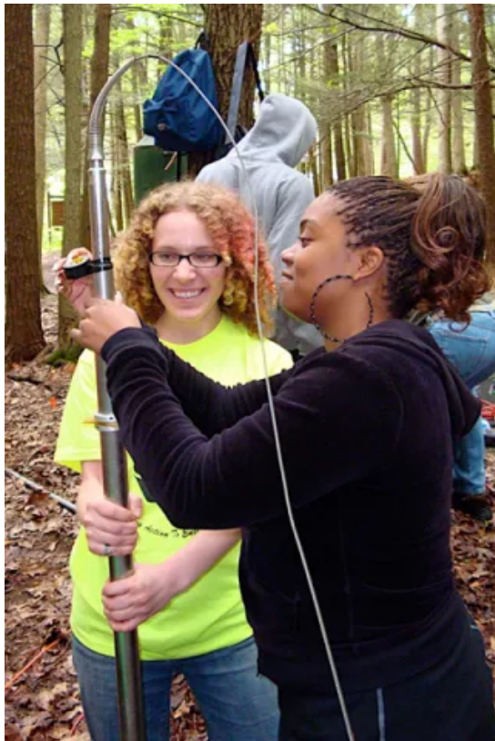
Claudia Shuman (left) and Stephanie Troutman prepare an optical televIEWER for deployment. They use the instrument to image fractures in the subsurface geology and estimate the fractures' orientation. Credit: Kamini Singha
