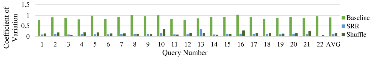
Fig. 17: Uncompressed TPCH - coefficient of variation of total instructions issued from each sub-core
