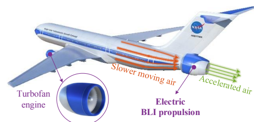
Fig. 3: STARC-ABL aircraft designed by NASA with a rear-mounted boundary layer ingesting fan [67].
