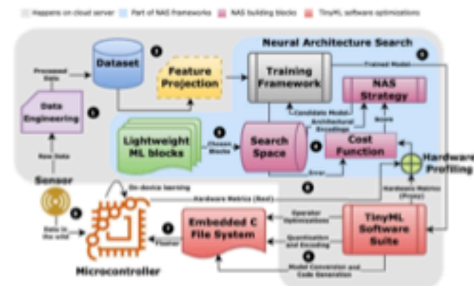
Fig. 1. Closed-loop workflow of porting ML models onto microcontrollers. Step (3)–Step (8) are repeated until the desired performance is achieved. (1) Data engineering performs acquisition, analytics, and storage of raw sensor streams (see Section III). (2) Optional feature projection directly reduces dimensionality of input data (see Section IV). (3) Models are chosen from a lightweight ML zoo based on the application and hardware specifications (see Sections VI and X). (4) NAS strategy builds candidate models from the search space for training and evaluates the model based on cost function (see Section VII). (5) Trained candidate model is ported to a TinyML software suite. (6) TinyML software suite performs inference engine optimizations, deep compression, and code generation. It also provides approximate hardware metrics (e.g., SRAM, flash, and latency) (see Sections V, VII, and VIII). (7) Embedded C file system is ported onto the microcontroller via command line interface. (8) Microcontroller optionally reports real runtime hardware metrics back to the NAS strategy (see Section VII). (9) On-device training or FL is used occasionally to account for shifts in incoming data distribution (see Section IX).
