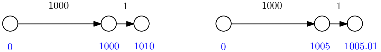
Figure 1: Example showing possible \alpha -approximate and smoothly \alpha -approximate distance estimates (estimates are blue). Note that in the \alpha -approximate case (left picture), the distance estimate can increase abruptly over a short edge. This is forbidden if the estimate is smoothly \alpha -approximate (right picture).
