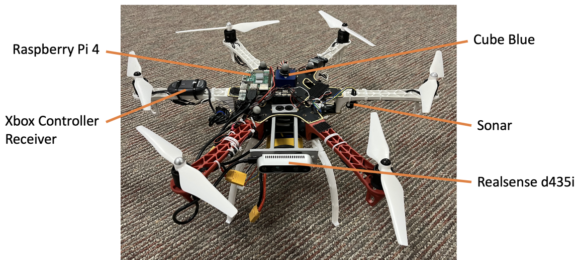
Fig. 1 Custom NIMBUS 550-size hexcopter outfitted with sensors used for REEF estimator evaluation.
