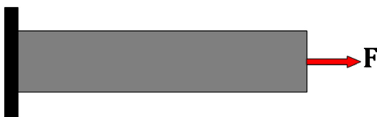
Fig. 7 Cantilever beam under axial load
