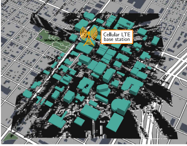
Fig. 4. Visualization of the cellular signal reliability map. The black regions indicate that the pseudorange bias due to multipath at the p th location exceeds a threshold \eta_{\max} = 0.5 m, i.e., b_{m,p} \geq 0.5 or there is no cellular measurement, i.e., b_{m,p} = \emptyset at the p th position. This figure is obtained with ArcGIS [49].
