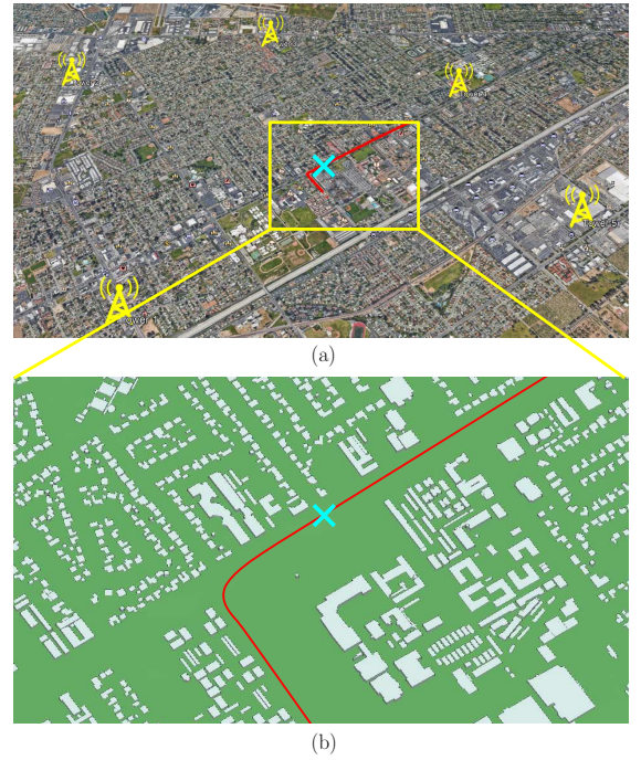
Fig. 2: (a) Simulation and experiment environment showing LTE tower locations and (b) 3D map of simulation environment. The receiver location is marked by an “X” for which the CIR is shown in Fig. 3. The vehicle trajectory is shown in red.
