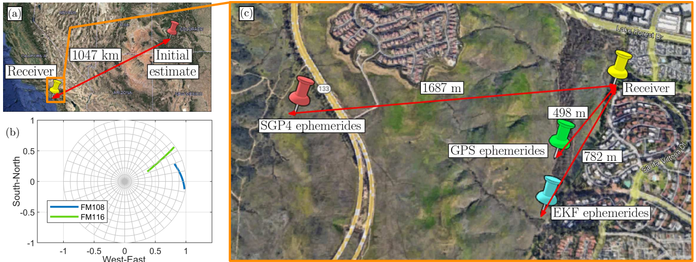
Fig. 8. Experimental results showing (a) the initialization of the NLS, (b) the sky plot of Orbcomm FM108 and FM116 SVs during the experiment, and (c) the final 2-D stationary receiver localization errors using (i) GPS-transmitted ephemerides, (ii) SGP4-propagated ephemerides, and (iii) closed-loop tracked ephemerides. Map data: Google Earth.
