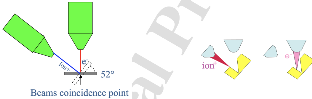
Figure 26: Schematic drawing showing the geometrical setting of a dual-beam FIB.
