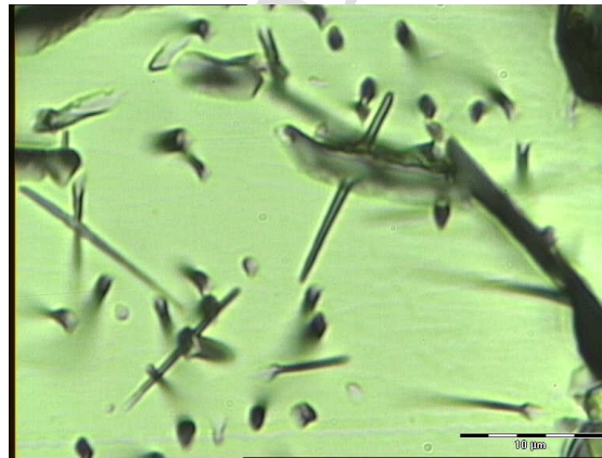
Figure 3: Etched spontaneous fission tracks in apatite visualized by optical microscopy. Apatite samples obtained from southern Uralides, Russia [93].
