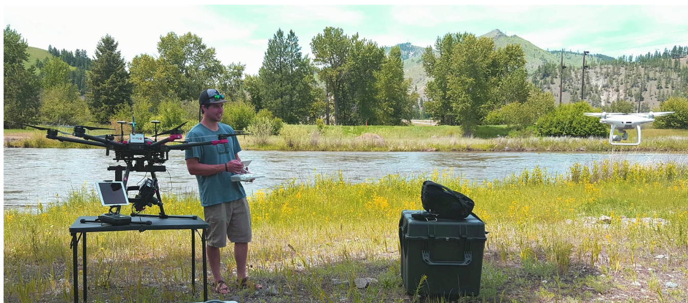
Fig 3. Image of drone being used to measure algal blooms in river.
