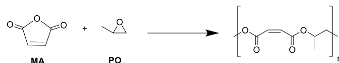
Scheme 5. Copolymerization of propylene oxide and maleic anhydride.
