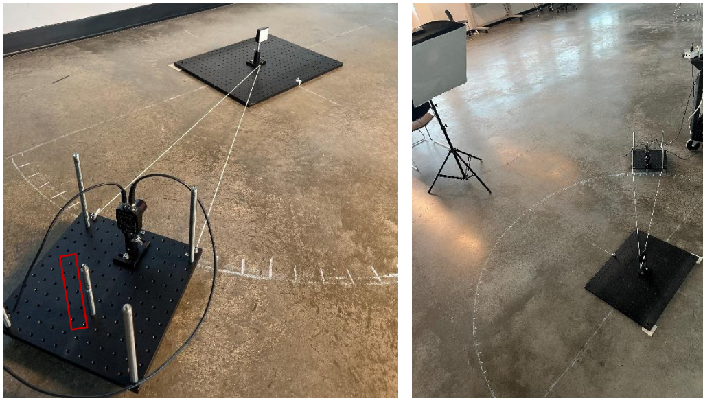
Figure 3. Setup for under-filled measurements. The necessary lens-source distance was greater than what could be achieved on our available optics benches, so we used a large area of a concrete lab floor. The post mounted behind the detector (red) was particularly
