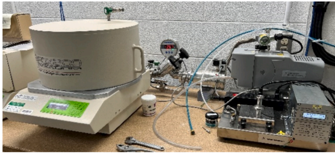
Fig. 2. Thermal conductivity measurement apparatus. (Left) FOX 200 Heat Flow Meter Apparatus enclosed in a sealed chamber. (Right) Vacuum pump.
