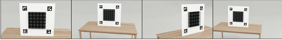
Fig. 8. Synthetic images rendered by Blender Cycle’s engine at four different camera positions. We set up a virtual scene and render camera captured images. In this way, we know the ground-truth camera locations, which allows us to evaluate our method’s tracking accuracy and compare it with the classic checkerboard-based approach.
