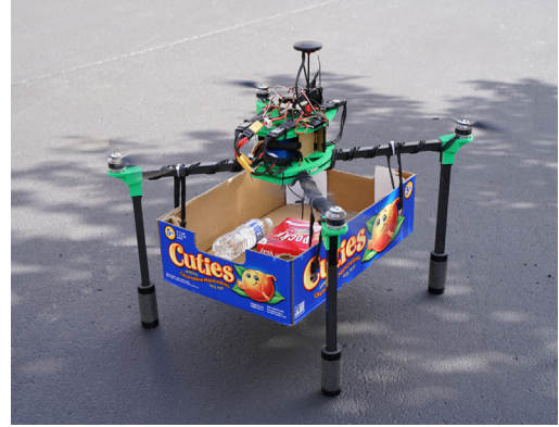
(b) A scaled-down prototype of the hypothesized quadcopter used in the simulation. This prototype is equipped with KDE3510XF-715 motors and has an empty weight of around 3 kg.
