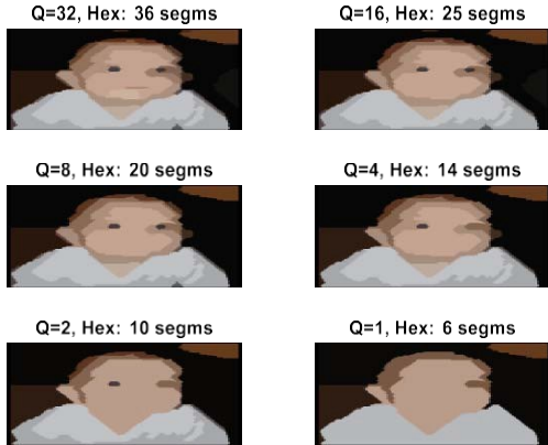
Figure 4: Segmented images using the sqL with 8-connectivity.
