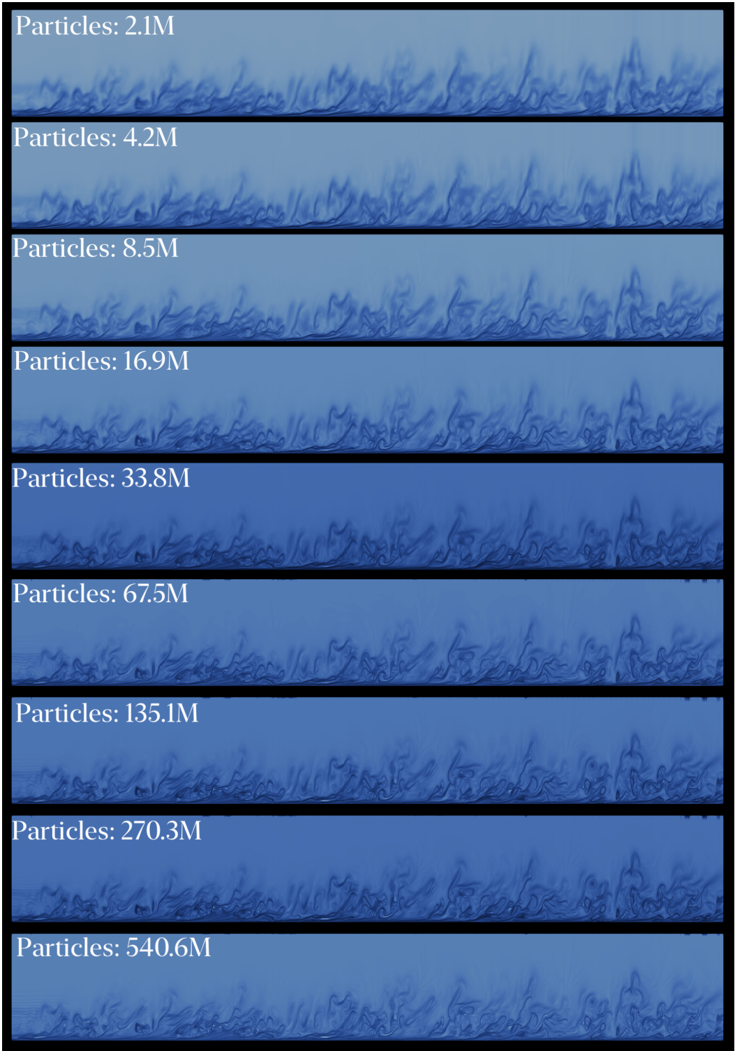
Figure 14. Attracting FTLE visualization as a function of particle count (HF: high temporal sampling frequency).
