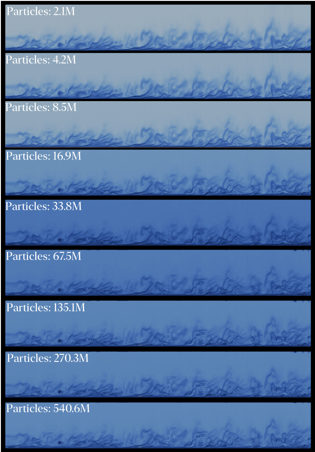
Figure 15. FTLE visualization as a function of particle count (LF: low temporal sampling frequency).
