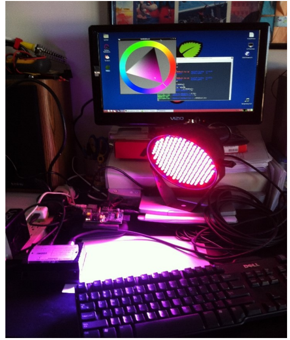
Fig. 2. Raspberry pi as a DMX light controller (adapted from [4])
