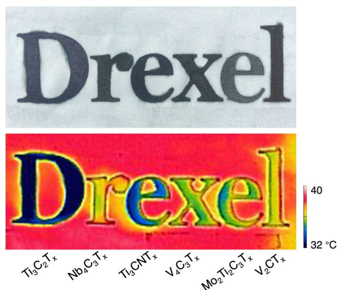
Fig. S12. Visible (top) and infrared (bottom) images of patterned fabric with different MXenes ( \text{Ti}_3\text{C}_2\text{T}_x , \text{Nb}_4\text{C}_3\text{T}_x , \text{Ti}_3\text{CNT}_x , \text{V}_4\text{C}_3\text{T}_x , \text{Mo}_2\text{Ti}_2\text{C}_3\text{T}_x , and \text{V}_2\text{CT}_x ) on a hot plate, showing the IR identification capability of MXenes.
