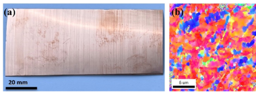
Fig. 5. Shear deformation processing of Cu a) FM strip of 105 mm width; and b) UFG microstructure in strip (RFN-TD thickness section) by EBSD.
