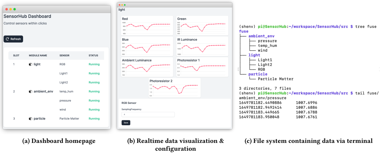
Figure 6: End user access via (a, b) web dashboard and (c) file system through terminal.
